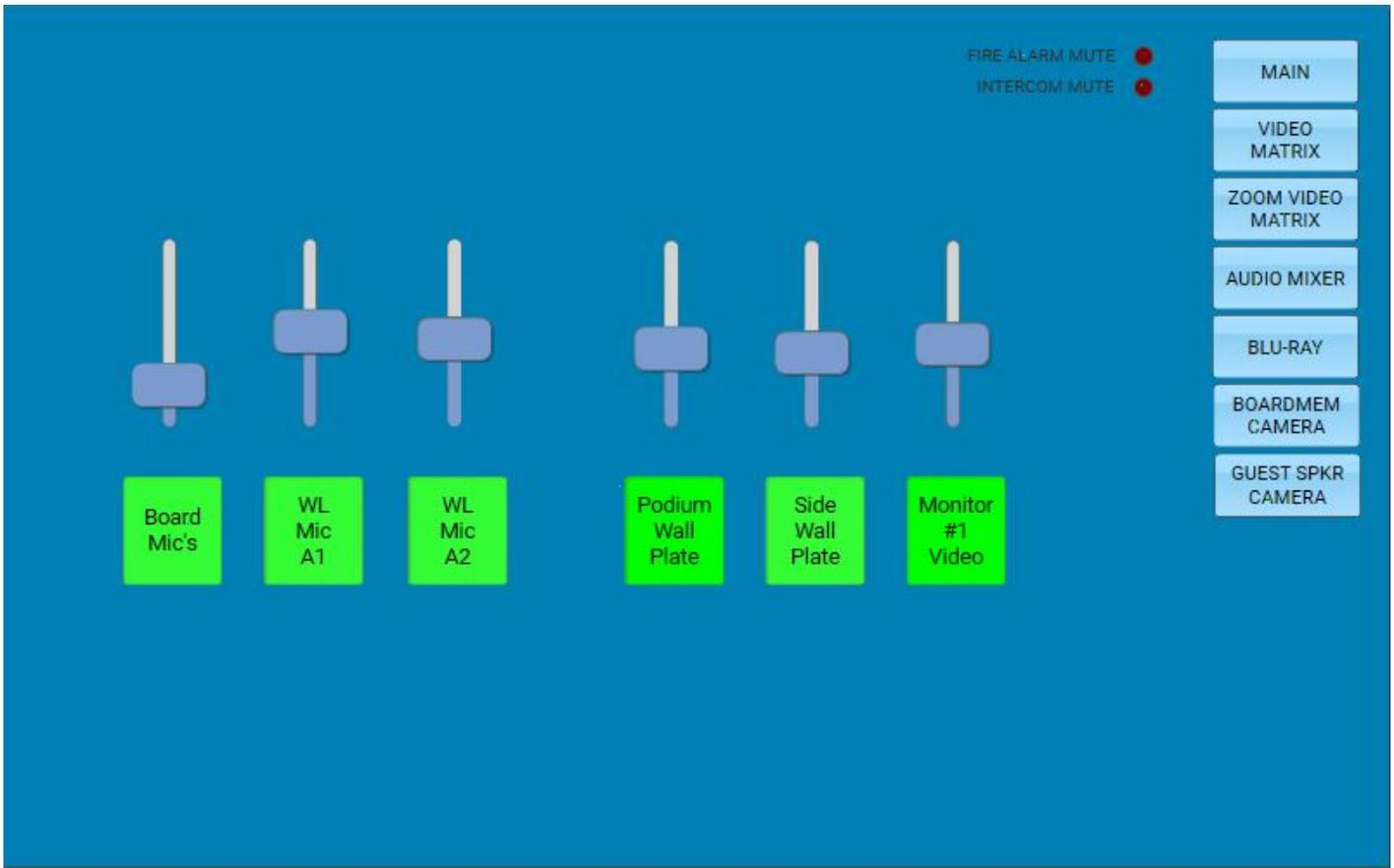
If you are using the ViewBoards to play a video without connecting a cable to the wall you will need to use "Monitor #1" as it is the only one with an audio out into the system. If plugged into the wall, the audio is received from the HDMI cable connected into the wall plate.
